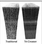
Tech-ni-Fold's "Tri-Creaser" is guarantee to totally eliminate fibre cracking
